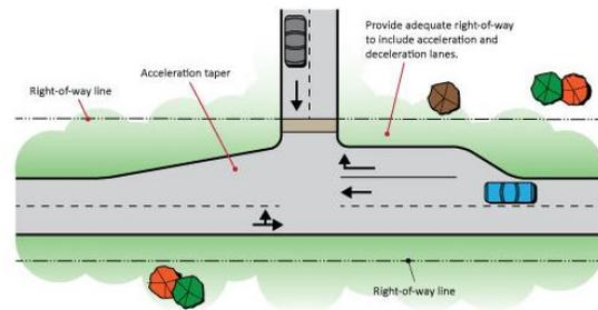
As shown in the above pictures, a right-turn lane forces the bike lane position to shift to the left, and these stressful lane configurations are part of standard road design practice in many parts of the U.S. The effects of left-turn lanes can be ignored since cyclists generally stay to the right of the road. Table 4.4 shows the proposed intersection LTS for signalized and unsignalized intersections.
