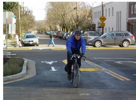
Lastly, **Bike Routes** are a series of connected bike facilities, often containing elements of both separated and shared bike facilities that promote bike mode share by use of route signs, wayfinding, and/or pavement markings.
